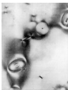
Figure 7 Formation of microcracks around impurities and bubbles in PC ( \times 25 ).
